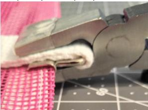
10 (b). **Optional:** Depending on the item or bag thickness--if you want to close clamp more snugly or evenly--you may be able to fold bag top around clamp back side then insert into pliers as shown, use firm, even pressure to make sure clamp is completely secure. Repeat on other strap end clamp.
