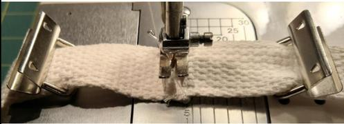
5. Turn length of strap over by twisting through clamp loop ends so raw seam allowance faces inside strap loop. Make sure clamp ends face same direction (both must be either up or down). Pull clamp ends outwards making strap loop flatten as a double layer of strap, as shown below.
