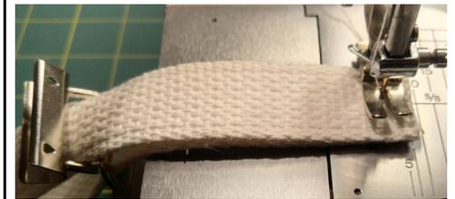
4. Finger press raw edges to one side or the other; topstitch raw edges down to one side.
